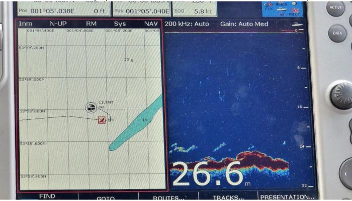
The screen of the GPS & sonar showing location, depth and 'picture' of the wreck Credit: Simon
