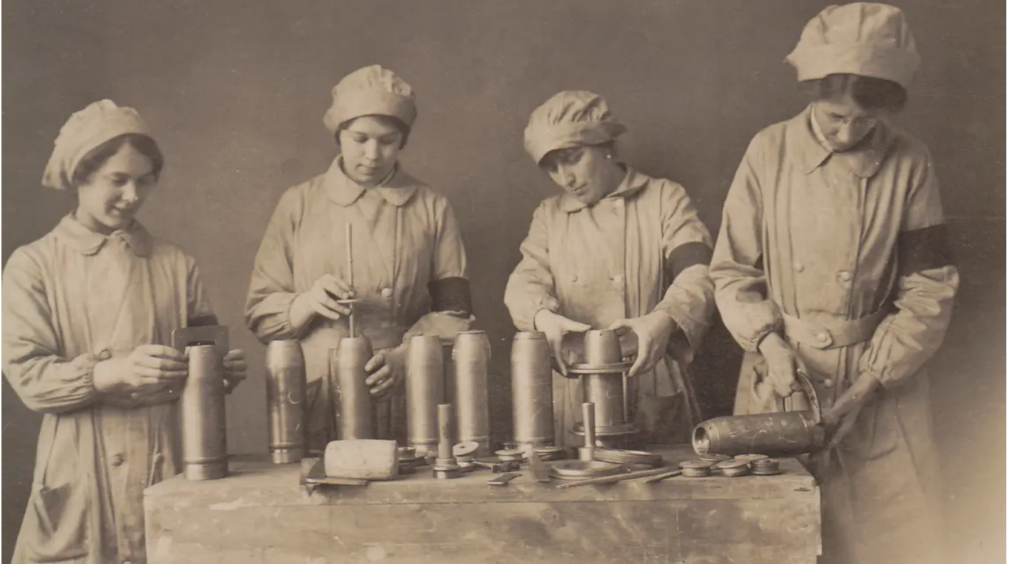
'Mmunitionettes' making shell casings at the Long Shop during the First World War Long Shop Museum
